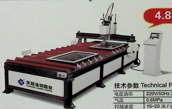
MD2-1500*2000(4000)-T 平移双工位全自动门窗打胶机 Automatic Door and Window Gluing Machine Translation Dual Station
